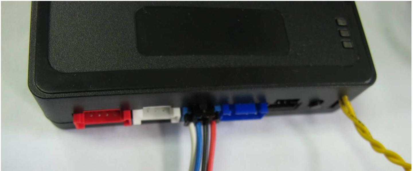
Or Cut the ATOM supplied connector with a knife as shown:
